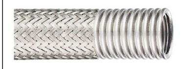
SB3 is a very high pressure corrugated stainless steel hose with a stainless steel braid. It has a higher pressure capacity than the standard braided metal hoses, along with high temperature capacity. It is resistant to bursting, cracking, and crushing even under very high temperatures and accidental exposure to flame, while being flexible and resistant to vibration. Applications include a variety of high pressure liquid and gas transfer. -320F to 1500F.
